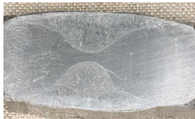
Submerged arc welded duplex stainless steel containing incomplete root penetration
