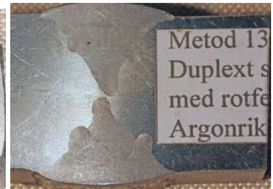
Incomplete root penetration were welds do not meet. Argon rich shielding gas
