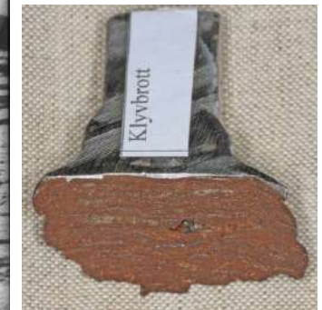
Fractured lifting device
