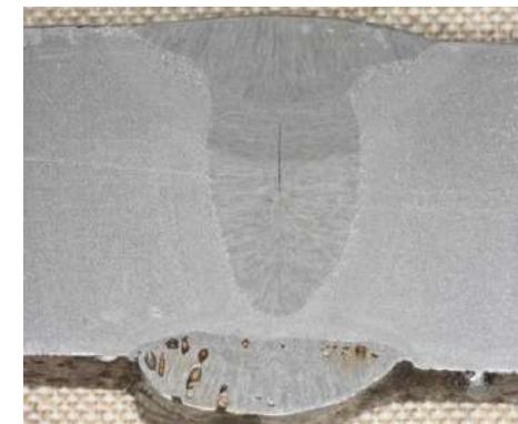
Solidification crack. Depth of the weld is greater than the width 8
