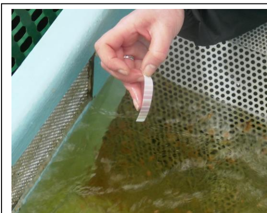
Routine pH monitoring with a probe is more typical than litmus paper.
