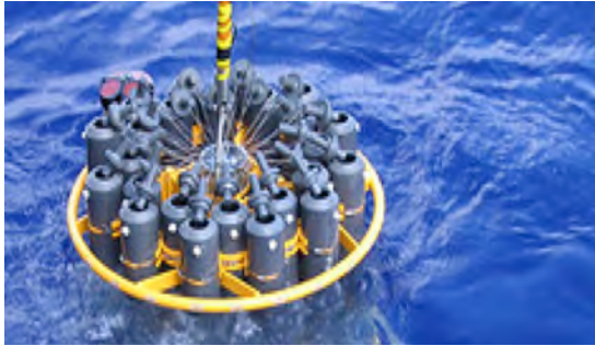
Sophisticated CTD devices can measure conductivity (to derive salinity) and depth
