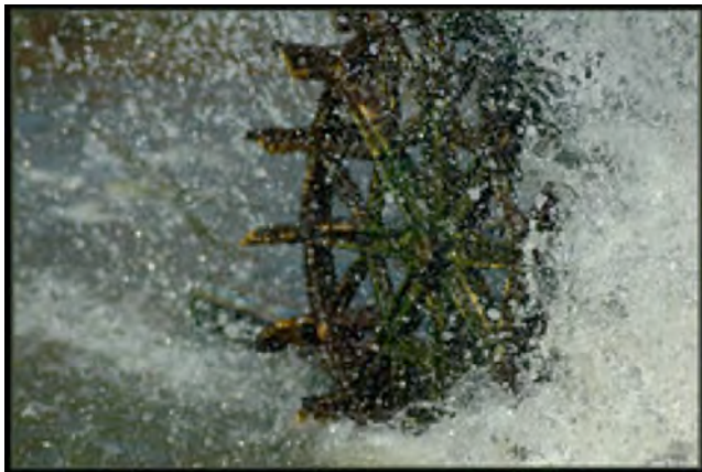
Surface agitation by a simple paddle wheel aerator is often enough to drive off supersaturated gases
