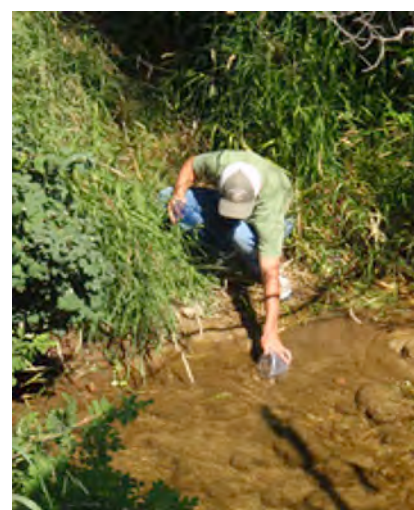
Collecting water samples for BOD testing
